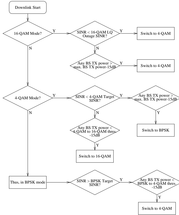
Figure 2.49: The AQAM mode switching algorithm used in the downlink of the CDMA based cellular network.
